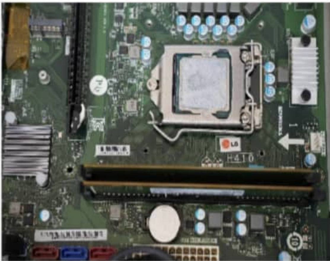
Figure 3.17: Apply the thermal paste on the CPU
